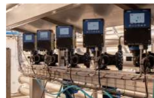
In-line injection of oenological products into grapes and juice from the bins
