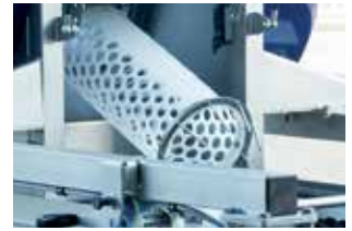
Oscillys 50 destemmer cage Short-length HDPE cage.
