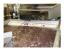
Hopper The harvest is poured into the hopper, and the liquid (juice, sugar water or clear water) is used for densimetric sorting.
