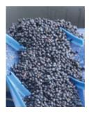
Berry elevator conveyor The conveyor takes the ripe berries to the top of the table. During conveying, the deformation of the belt improves the draining of the berries by limiting crushing.
