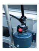
Hydraulic pump This pump makes it possible to tilt the belt according to its use.
