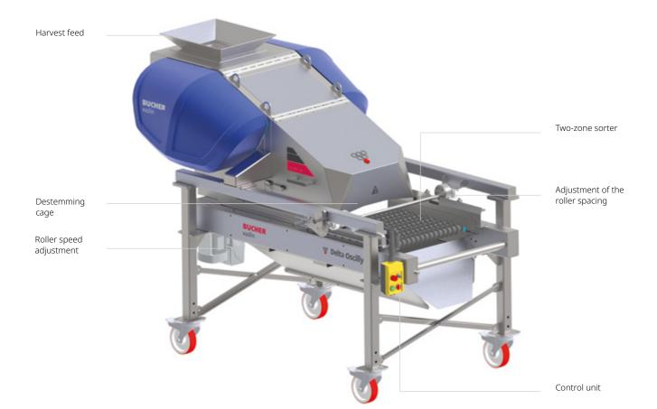
Drainage tray With adjustable roller spacing. Additional cage DN 25, 30 or 35. Cage 1st mounting Choice of 30 or 35 mm. Frame for Delta TRV 20 Height between 1000 and 1500 mm.
