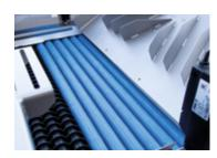
Vibrating distribution hopper The harvest is conveyed to the distribution rollers.
