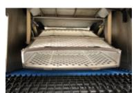
Oscillys XM/XL destemmer cage Wide cage and pentagonal shape ensures treatment in the central zone and in a single layer of bunches. The kinematics of the cage generate a
